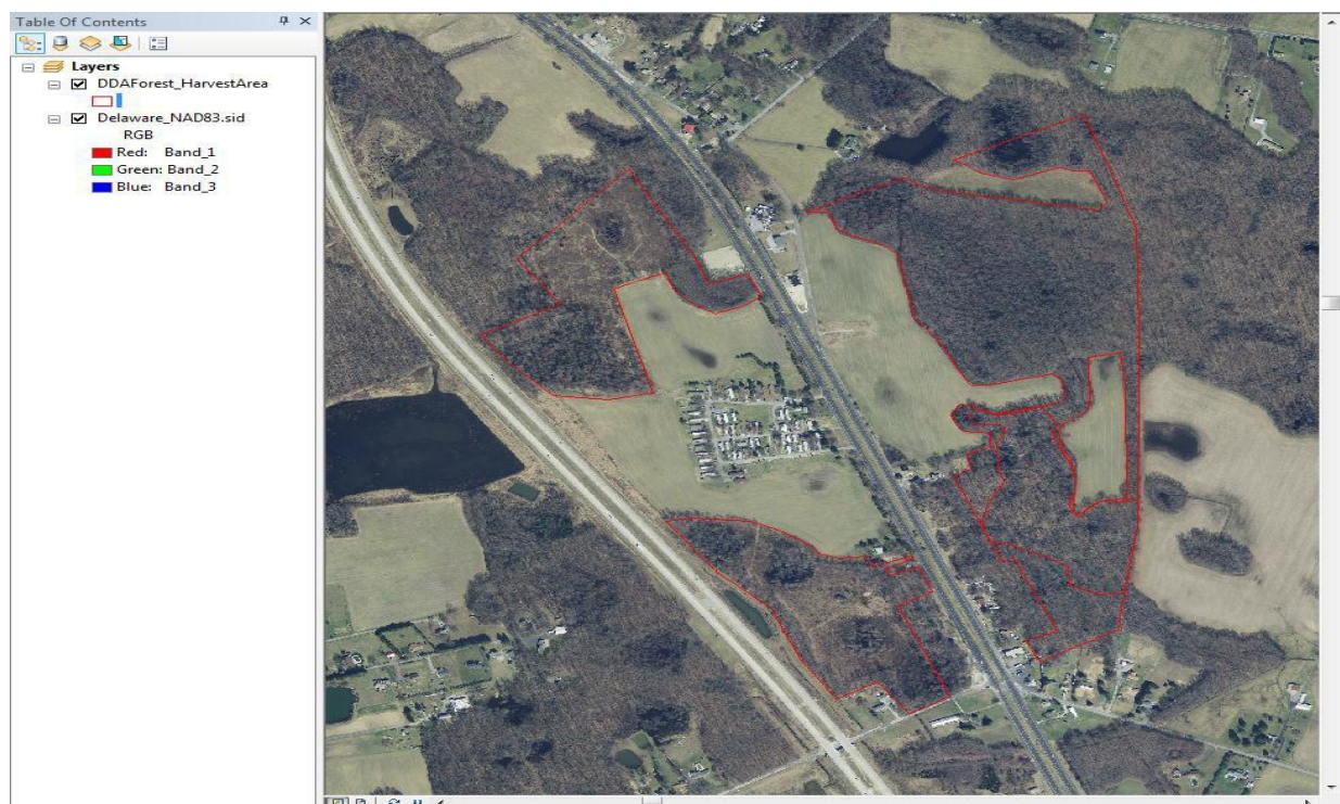
Figure 1: The ArcMap layer “DDAForest_HarvestArea” contains the shapefiles of harvested forest, indicated by the red outlines.
