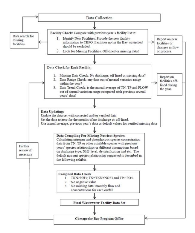
Figure A-1. Wastewater facility nutrient data processing flow diagram (source: USEPA 2016).
